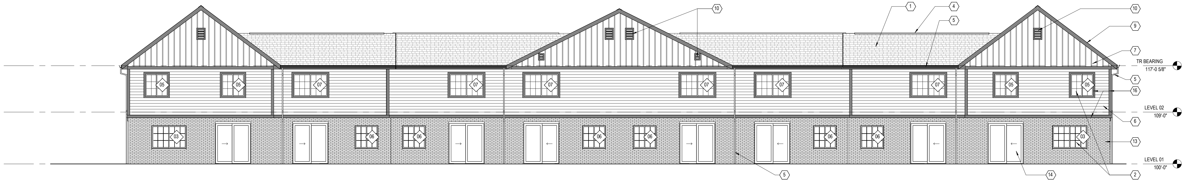
2 ELEVATION BLDG TYPE A (BLDG #1, 2, 10 & 11) REAR 1/8" = 1'-0"
